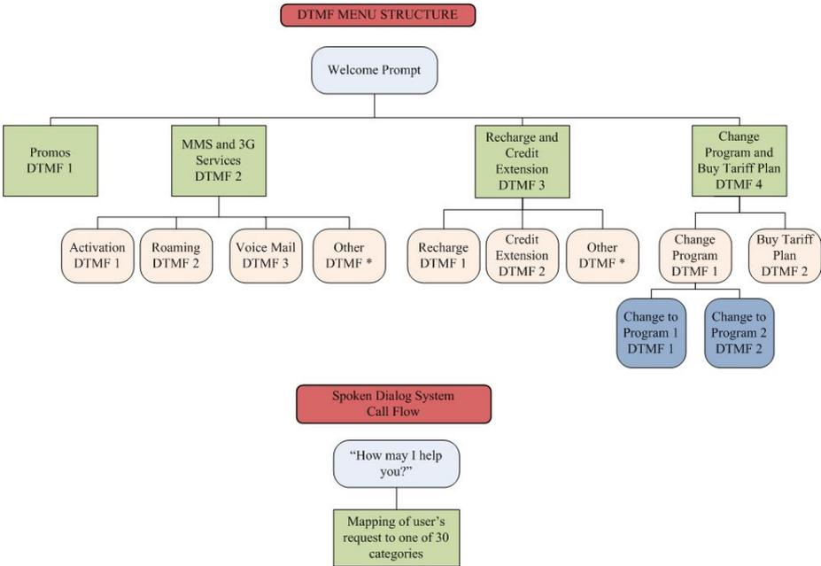
**Fig. 3.** DTMF and Speech-based dialogue systems basic architecture. Optimal tree traversal is faster for the former. Error handling, universals, help sub-dialogs in the Spoken Dialog system and some sub-menus in the DTMF system are excluded for ease of presentation.
